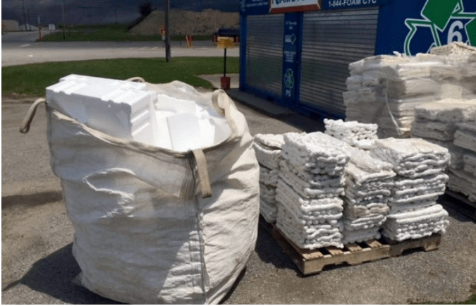
Styrofoam is compressed into densified ingots.
