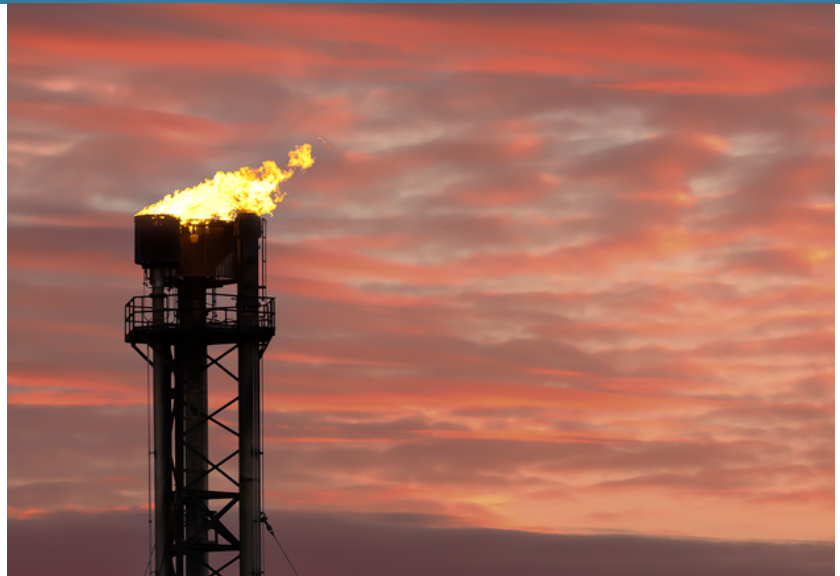
Methane flaring is the intentional burning of excess natural gas at processing facilities. Photo Source: Adobe Stock.
